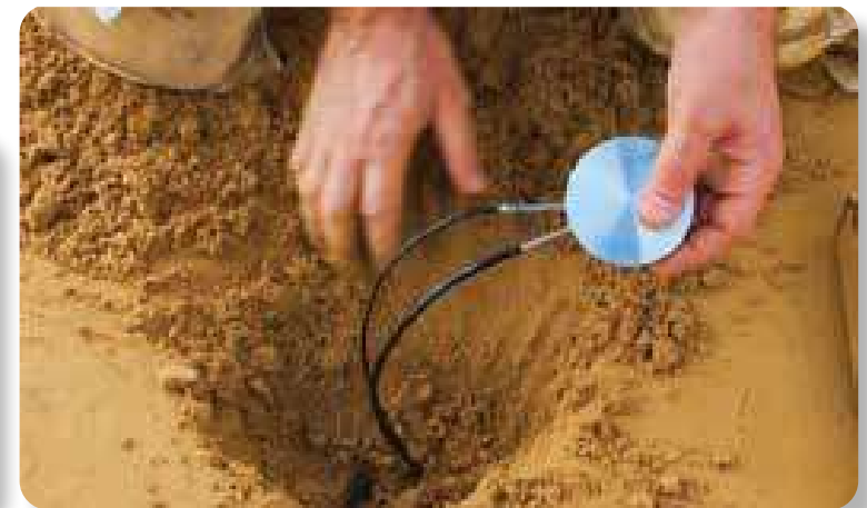
Load measurement sensors positioned at the top, bottom and sides of the pipe
